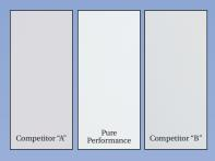
**Brightness Test Method:** The reflectance (i.e. brightness) of each coating was evaluated according to ASTM D 2805-88.
